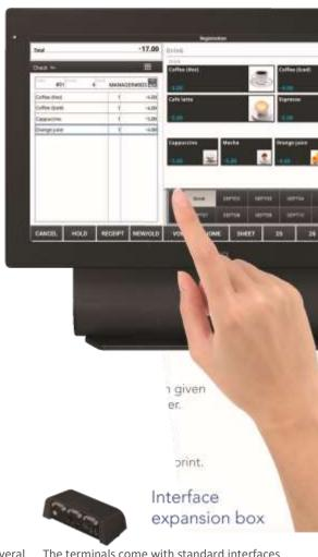
LAN-compatible model compliant with IEEE802.11a/b/g/n (the V-R7100) that further increases freedom in installation. The elimination of network cables makes it easier to use the V-R7100 in pop-up retail stores, exhibition sites and other temporary locations.
